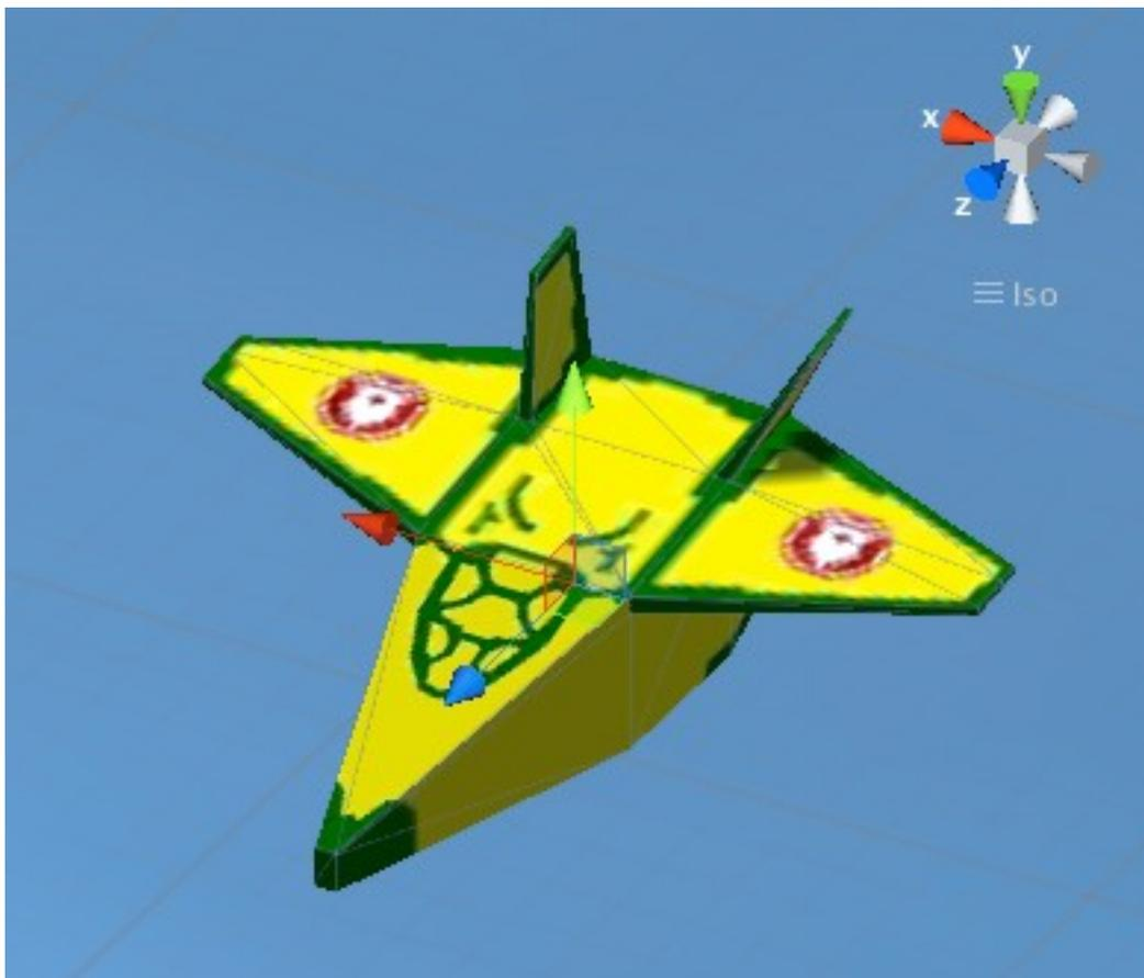
The ship's axes must be aligned so that Z points forward, X to the right and Y up. If your mesh's axes are not aligned this way, then there is an option to spawn and attach the mesh as a child object to the controller (which is the preferred method). See the **Mesh Child Or Prefab** property on the ship's controller component.
